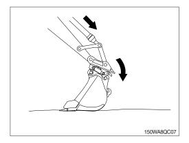
(10) To engage the quick coupler, release the quick coupler button on the right joystick lever.
