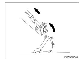
(9) To lock the quick coupler, release the quick coupler button on the right joystick lever.
